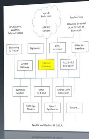
IGate stations allow communication between disjoint radio networks by allowing some content to flow between them over the Internet.
