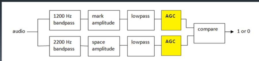
With either mismatch case, the demodulator has a difficult time rapidly deciding which tone is stronger and it is less reliable.
