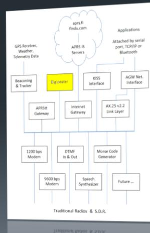
A digital repeater serves the same purpose as a voice repeater. It allows communication between stations that can't hear each other directly.
