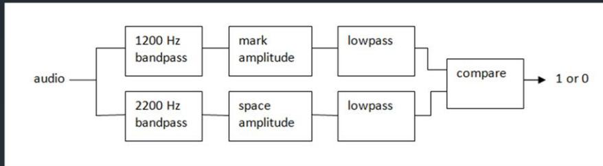
This is one way we can implement a demodulator for AFSK. We start off with a bandpass filter for each of the audio frequencies. In the old days, you might use an inductor and capacitor. Later we progressed to active filters with op amps. Today it can be done in software.
