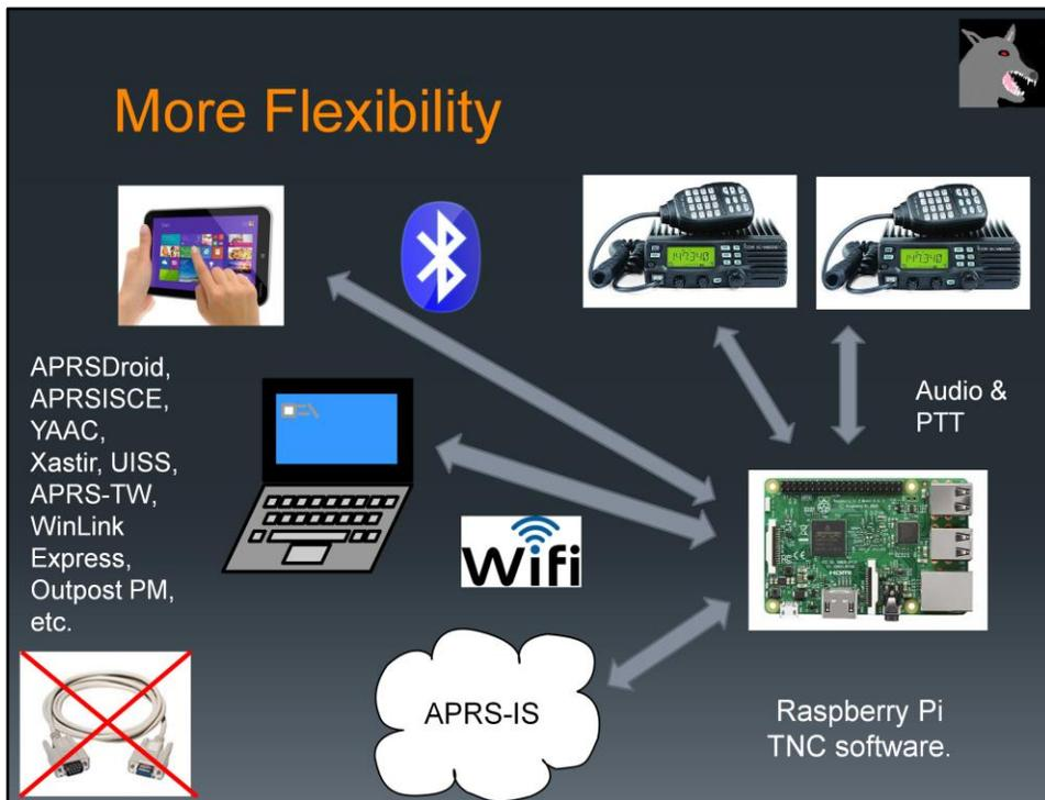
The software TNC approach is very flexible. You are no longer constrained by that serial port cable and a single radio interface.
