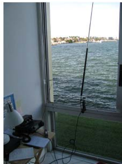
Operators Position and 6-2m Antenna
