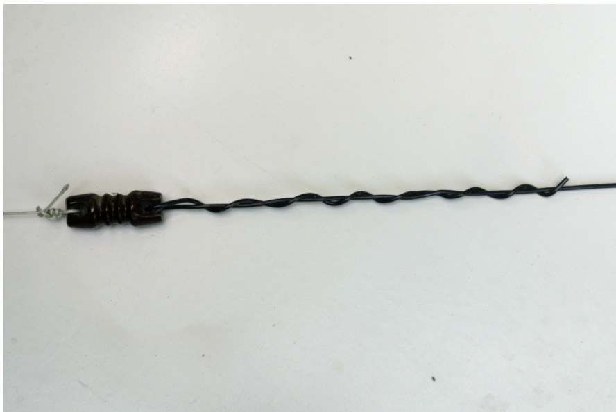
Radial with Extra Wire for Tuning – Support Cord is on the Left
